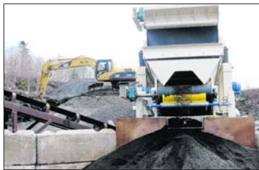
In addition to recycling tear-off shingles and using the material in their hot mix asphalt, Ocean has also begun putting reclaimed asphalt pavement materials into their mix.
