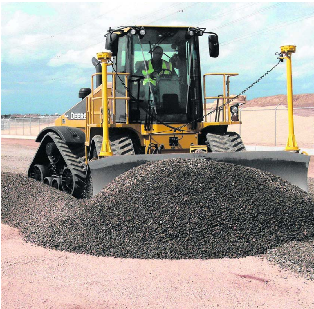
The 764 HSD finishes grades and does up to twice as fast as a traditional crawler. Its articulated-frame steering and four-track oscillating undercarriage make the 764 HSD highly manoeuvrable, reducing the need to transport it on trailer for short distances.
